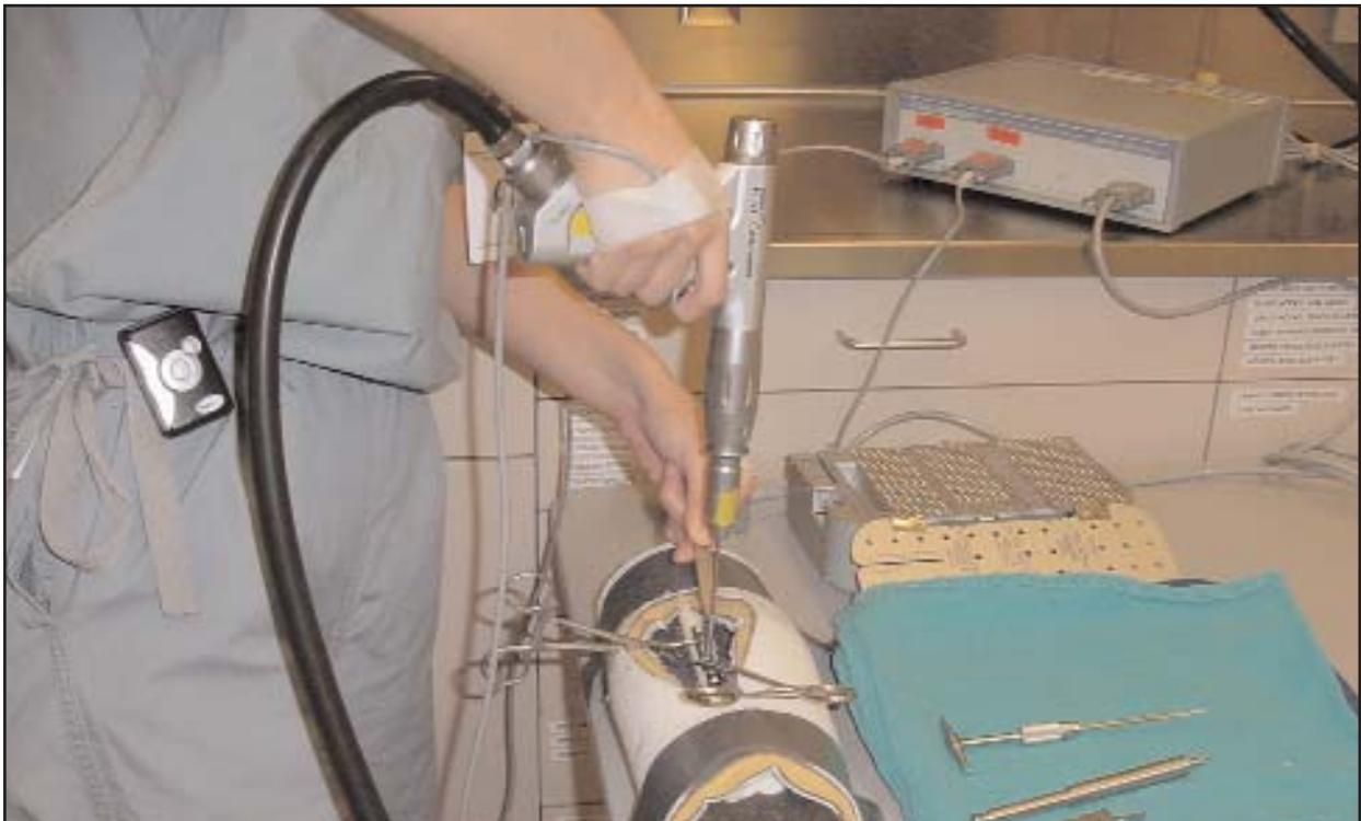
As part of a research study, a student practices bone drilling and plating using a hand motion detector, which analyzes his movements.
